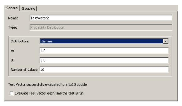
Gamma uses the function gamrnd and takes parameters for A and B.
