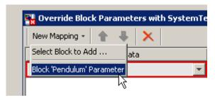
In the override table, the **Simulink Data** field shows that this entry is linked to the Pendulum block but the question mark (?) indicates that no parameter for the block has been mapped.
