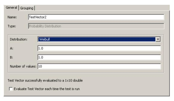
Weibull uses the function wblrnd and takes parameters for A and B.
