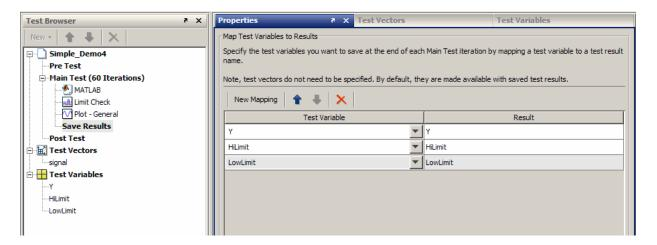
After specifying which test variables to save as test results, specify the name of the MAT-file to use. Using this MAT-file you can reload the test results into the base workspace. By default for a test that is untitled, the SystemTest software names the file Untitled\_results.mat and puts the file in the same folder as the TEST-File. To change the name or location of the MAT-file, click the test name in the **Test Browser**, then click the **Output Files** tab in the **Properties** pane.
