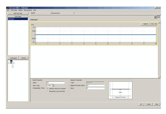
The example model has two Inport blocks, which appear in the signal list in the Test Case Editor. In1 is selected here and you can see that the signal was created using the same **Data Type** for that signal as the Inport block had in the model, **double** in this case.
