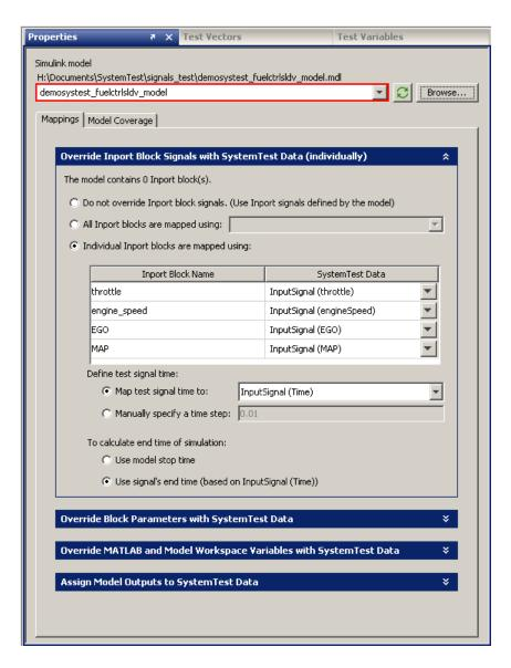
When the test is executed, the Simulink element will test the model using the Inport block signals mapped from the spreadsheet.
