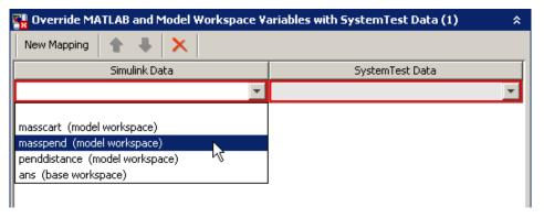
3 Specify which SystemTest test vector or test variable you want to map to the Simulink workspace variable. Click the **SystemTest Data** field of this row to see all available test vectors and test variables. For this example, select **pend**.
