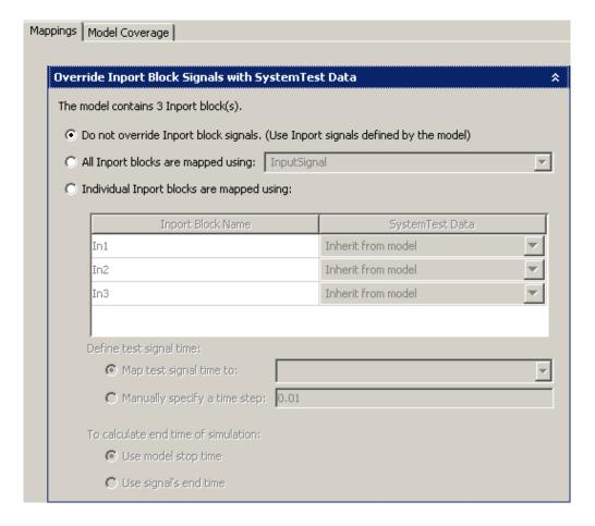
The first option, **Do not override Inport block signals**, is selected by default. That means the test will run the model without modifying any Inport block settings. Any data the Inport blocks are configured to use will be used during execution. If you want to override the model, use one of the other two options.
