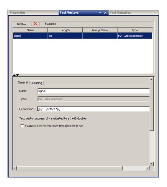
After you create the test vector, in the **Test Browser** pane, the **Main Test** section label updates to include the number of iterations defined by the test vector. It should say Main Test (60 Iterations).
