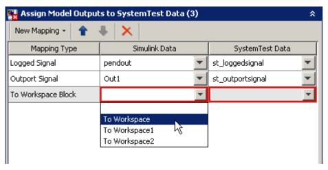
3 Specify the SystemTest test variable to which you want to map the To Workspace block. Click the **SystemTest Data** field and select a test variable from the list. For this example, select **New Test Variable** to create a test variable.
