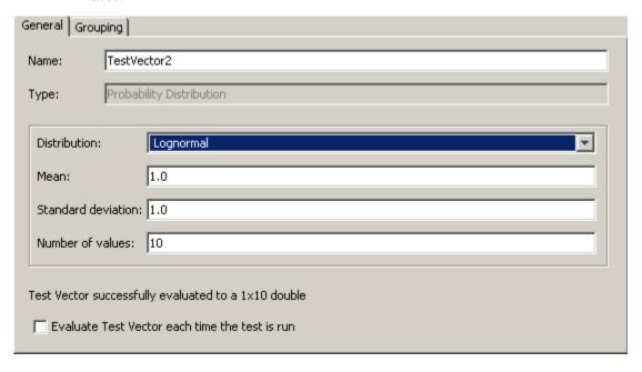
Lognormal uses the lognrnd function and takes parameters for **Mean** and **Standard deviation**.
