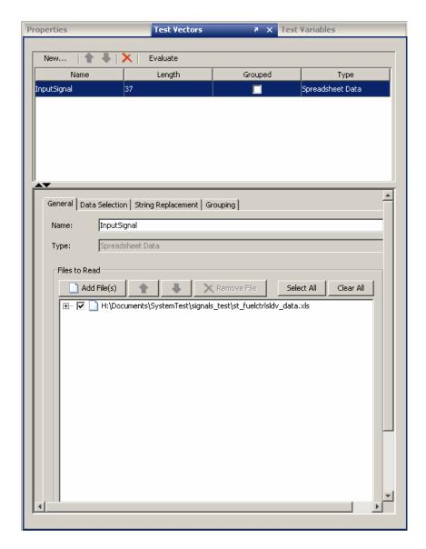
Now that the test vector is set up, you can set up the Simulink element to override the Inport blocks using the test vector values from the underlying spreadsheet file.
