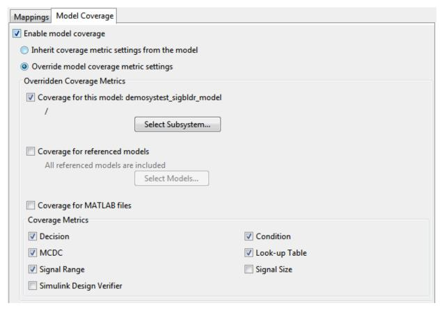
8 Click the **Select Subsystem** button in the **Overridden Coverage Metrics** section to specify the root model of your coverage data. Make your selection in the System Selector dialog box and click **OK**.
