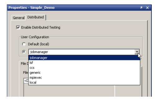
User configurations contain other information in addition to scheduler selection, and are used to define other distributed computing parameters. See Programming with User Configurations in the Parallel Computing Toolbox documentation for details on setting up the user configuration.
