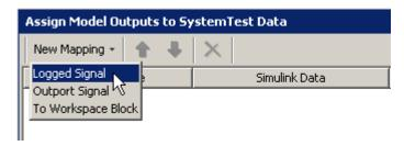
2 Specify the signal you want to capture. Click the **Simulink Data** field to see all the signals in the model. For the Inverted Pendulum example, select **pendout**.
