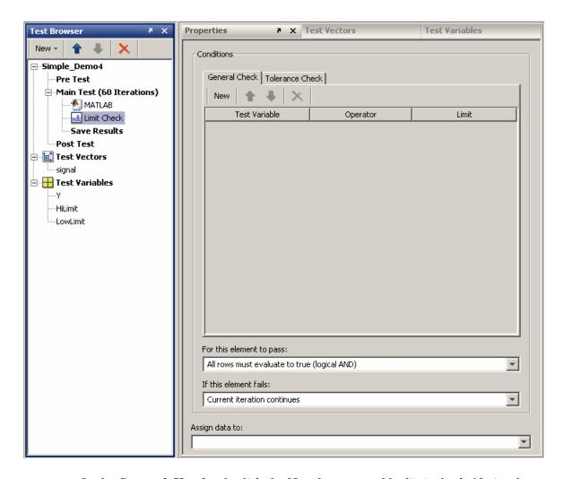
In the **General Check** tab, click the **New** button to add a limit check. Notice that the Limit Check element icon in the **Test Browser** shows a red x, which indicates that information is missing. The corresponding red outlining in the **Properties** pane highlights any fields that require configuration. A test cannot run unless everything is properly configured.
