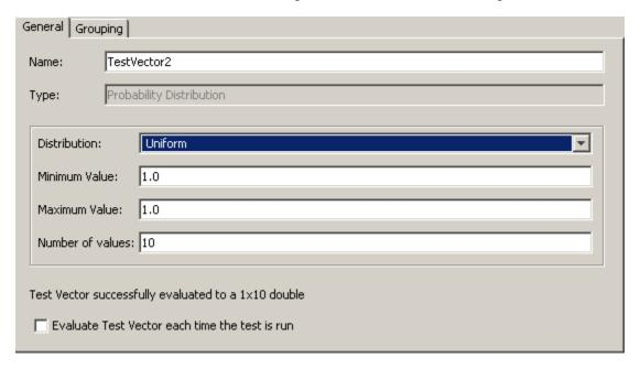
Uniform uses the function rand and takes parameters for **Minimum value** and **Maximum value**. The SystemTest software uses the following calculation for uniform:
