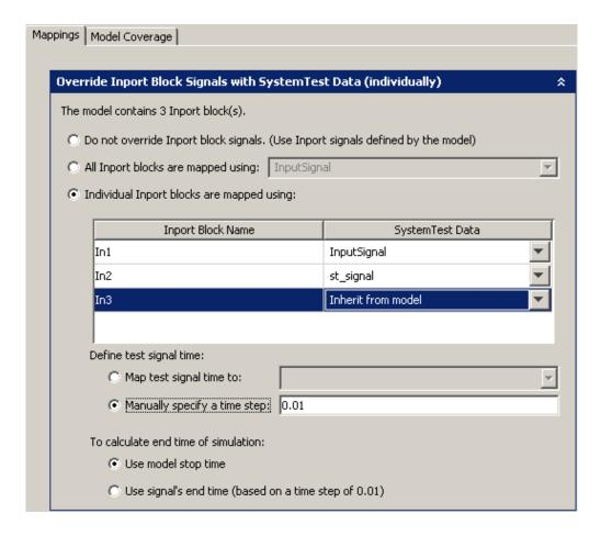
When you select this option, the mapping table becomes editable. In the case shown here, In1 and In2 are being overridden with SystemTest data, and In3 is using the value in the model.
