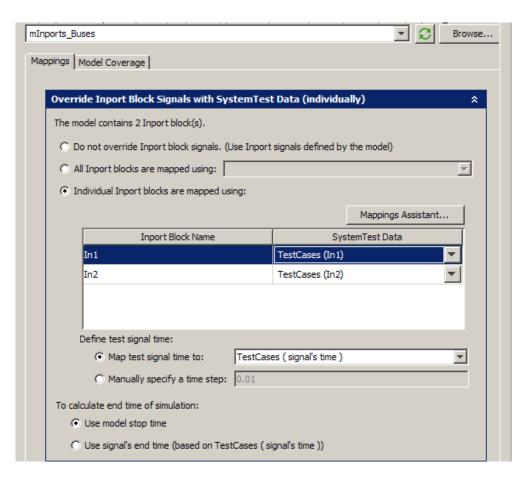
TestCases (In1) is the signal called In1 in the Test Case Data test vector called TestCases. In1 is a regular signal and In2 is a bus signal. You can see that it is a bus if you expand the signal in the **SystemTest Data** list.
