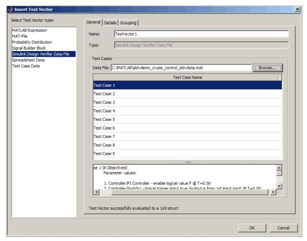
To see information from the Simulink Design Verifier data file, click the **Details** tab. This provides analysis information on the data file, and the model Inport blocks associated with the test cases. If the test cases involve any model parameter configurations, they appear in the **Parameters** section. This section will list any parameters that are used as part of a test case. The information in this tab is not editable.
