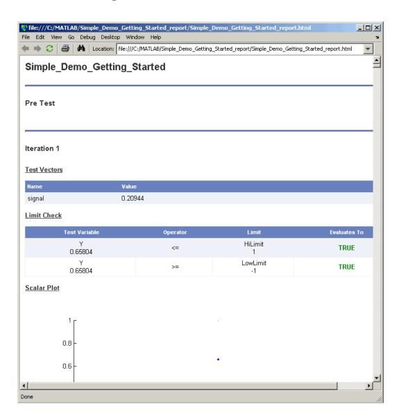
The Main Test section of the report shows each iteration. You see the value of the test vector signal and determine the values the Limit Check element used in evaluating whether the test passed. For the first several iterations, the value of Y did not exceed either the high or low limits so the iterations passed. You can also see this in the scalar plot drawn while the test ran. For other iterations that failed, you can scroll through the report to find the values of Y.
