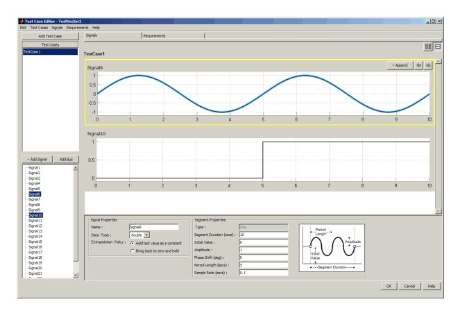
In the lower-left pane is a signal list that lists every signal in the selected test case. You can click signals in the signal list to select or clear them. You can select multiple signals by using the **Ctrl** key as you click on them.
