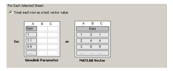
In the first case shown here, column A contains values for the parameter Gain. Suppose this column contains 10 values, in rows 2 through 11 (row 1 is a header). The resulting test vector would be a 1-by-10 array containing 10 values. The first value is 1, the second value is 1.1, etc. The ten populated rows result in a total of ten values, each row being one scalar value.
