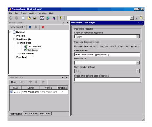
To see the resources you created for communications with your two instruments, click the **Resources** tab at the bottom of the SystemTest window. You can see the **Generator** and **Scope** resources, along with their GPIB settings.
