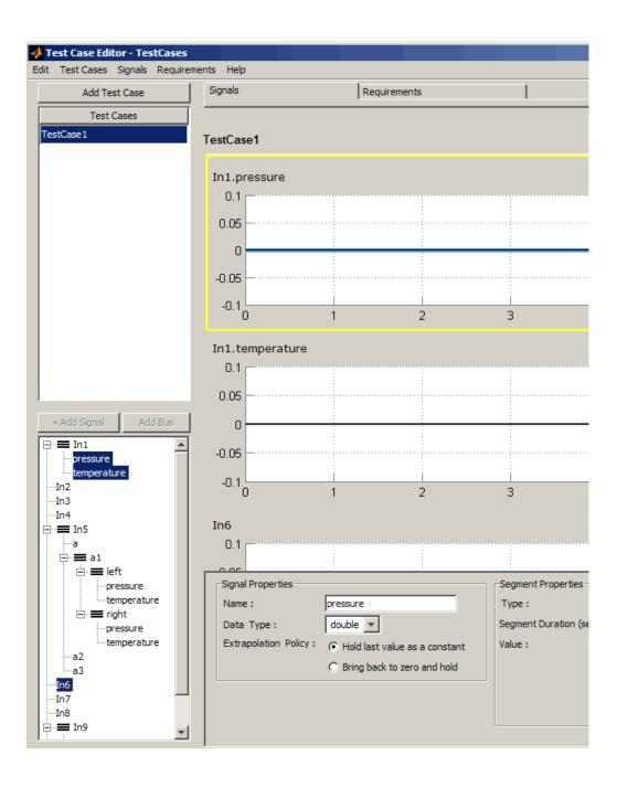
**Note:** If you have a model that contains buses, you can automatically generate a test harness from the model. It will create and configure all of the appropriate parts of the test, including elements, test vectors, and mappings, and create a test case containing all of the Inport blocks as buses and/or signals. For more information, see "Test Harness Generation" on page 6-2.
