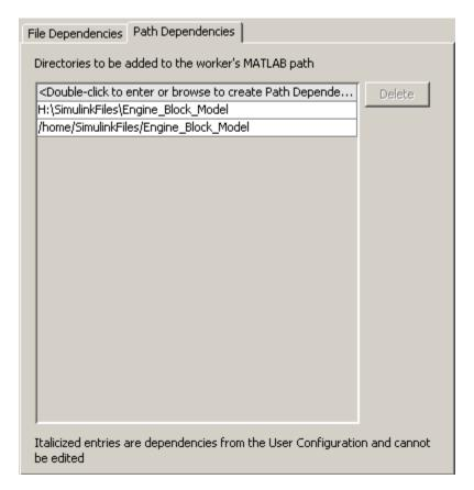
Notice in this example that the path is listed twice, once in Windows® format and once in UNIX® or Linux® format. If you have a heterogeneous cluster that contains both Windows and UNIX or Linux worker machines, you need to add the path twice so that all workers can use it.
