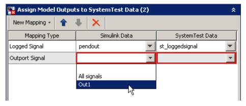
3 Specify the SystemTest test variable to which you want to map the outport signals. Click the SystemTest Data field and select a test variable from the list. For this example, select st\_outportsignal.
