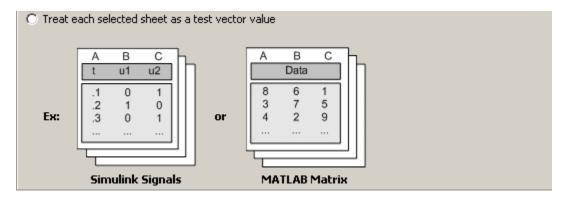
If the sheet contains multiple rows and columns, the resulting test vector value is a matrix. In the first example shown here, labeled Simulink Signals, this spreadsheet file contains 3 sheets. Suppose each sheet contained the three columns shown, t, u1, and u2, and had just the three rows of values shown. The resulting test vector would be of length 3 since each sheet is one test vector value and there are three sheets, and each of the three test vector values would be a 3-by-3 matrix.
