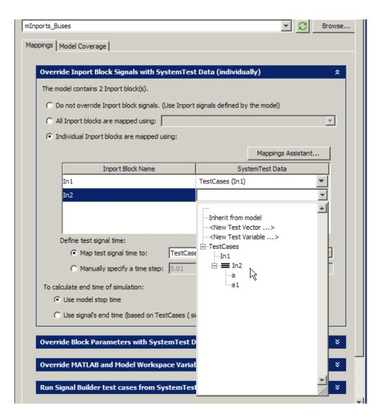
The Simulink element is configured to map the signal time to the test vector signal's time and to use the model stop time.
