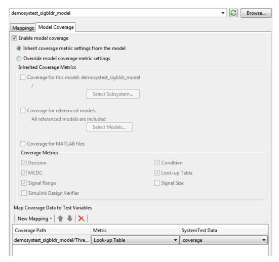
5 If you want to use the model coverage settings you already have on the Simulink model, select the **Inherit coverage metric settings from the model** option. Then go to step 12.
