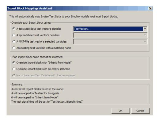
When you click **OK** in the Mappings Assistant, the signals are entered into the **SystemTest Data** column in the table, and the test uses the signals' time by default.
