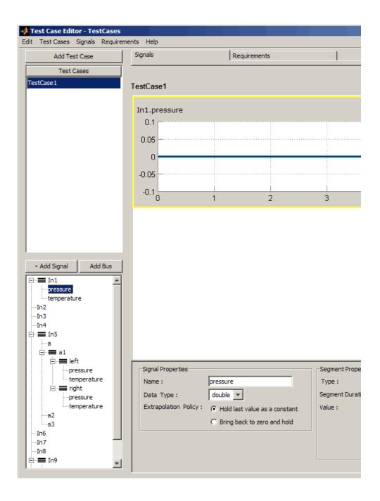
In this example you can see that In1 is a bus containing two signals, pressure and temperature. The signal pressure is selected in the signal tree and consequently is displayed and selected in the editing pane, when in the Edit view.
