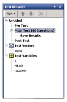
2 Specify the element you want to add to the test section. For this example, click the New > Test Element button and select MATLAB. A MATLAB element appears in the Main Test section of your test and the MATLAB element property page opens in the Properties pane of the SystemTest desktop.
