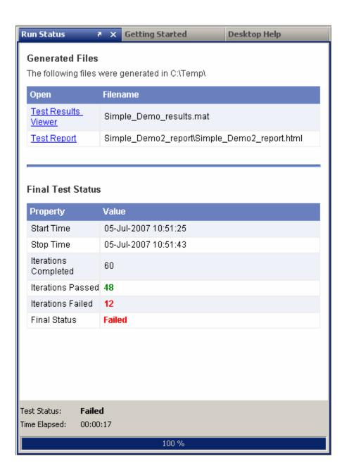
If your test includes a Plot element, the SystemTest software creates the plot and updates the plot during each iteration. Since Limit Check elements evaluate whether an iteration passed or failed, they directly affect the data that appears in the Test Report and the **Run Status** pane.
