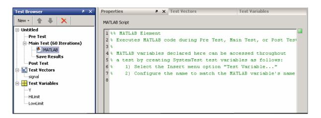
3 In the **Properties** pane, type the following code in the MATLAB Script edit box. This MATLAB code calculates a value for Y that is dependent on the test vector signal.
