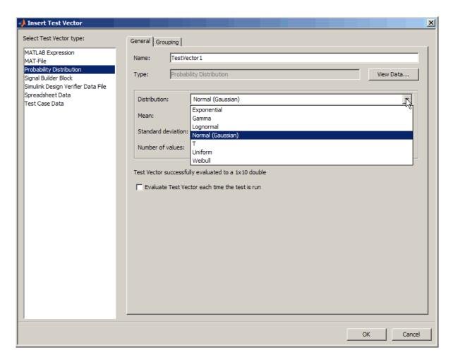
If you have the Statistics and Machine Learning Toolbox software, all of the functions shown in the figure appear in the list. If you do not have this toolbox, you can use normal (Gaussian) and uniform.
