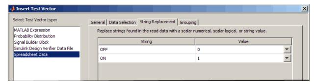
If you want to map the same strings to different values, you have to create separate test vectors and do each replacement mapping separately. For example, in the previous case, you might want the values for Switch A to map to 1 and 0 as shown, but for Switch B you might want to use 100 and 0. In this case, create a test vector that reads only column A and replace ON and OFF with 1 and 0, and then create a second test vector for column B that maps Switch B values to 100 and 0.
